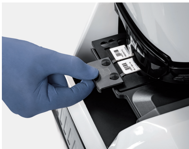
2 Loading device with 2-slide tray
